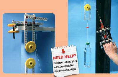
But you can achieve an even greater savings in force. The more pulleys the combination pulley has — more accurately, the more strings there are running to and fro — the more force you save. The load is simply divided by the number of strings.
