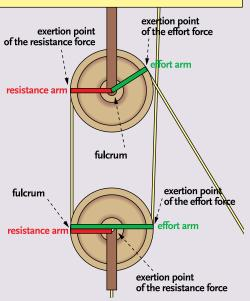
Combination pulley: a combination of a fixed and a movable pulley.
