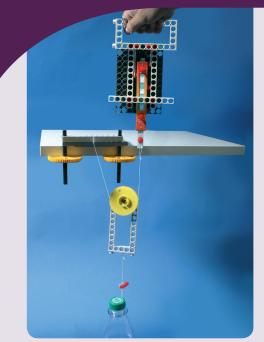
This is how we measure force with the movable pulley.
