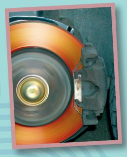
brake pedal to the main cylinder. From there, the braking force is transferred equally by separate pathways to the braking cylinders on the wheels. Big and heavy vehicles, e.g. a tour bus or dredger, have so-called servo brakes, which amplify the braking force through a pump.
