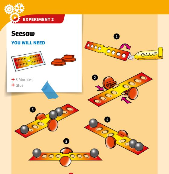
A seesaw will tip downward on the side with the greater weight. Both the weight of the objects on the seesaw and their distance from the center fulcrum point are important. The farther a weight is from the fulcrum, the greater its effect, or force.
