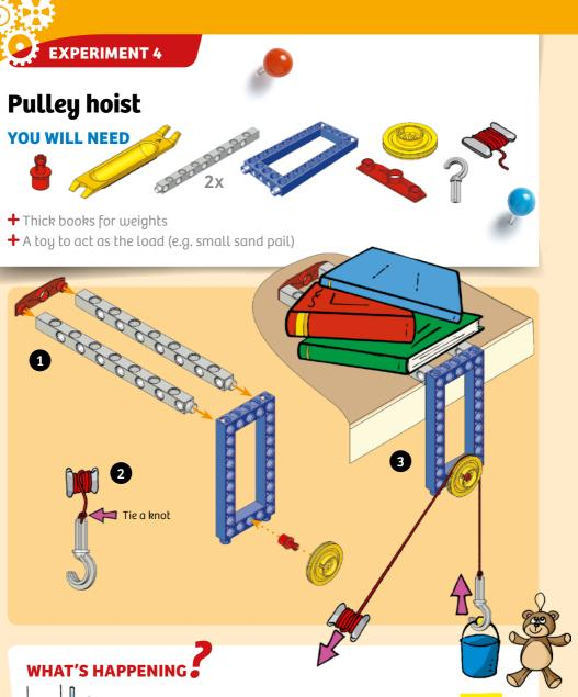
By pulling down on the string, you lift the bucket up. The pulley changes the direction of the force. Normally, you have to pull upward to lift something up. This pulley doesn't reduce the force needed, but it is still a helpful tool. For example, a painter can use it to lift a bucket up to the top of his scaffolding.
